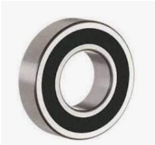
FAG (Schaeffler) 6215-2RSR-C3 Radial/Deep Groove Ball Bearing - Round Bore, 75 mm ID, 130 mm OD, 25 mm Width, Double Sealed, C3 Internal Clearance
